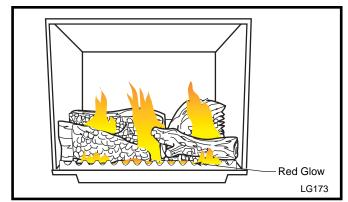
Fig. 33 Correct burner flame pattern.
